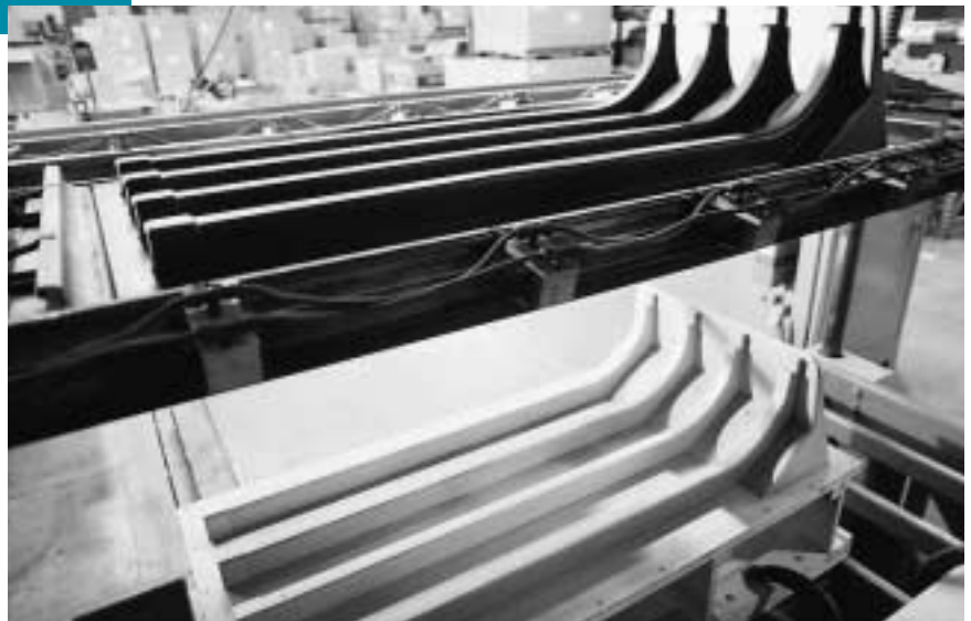
Figure 8 Thermoformed Part Designed with Ribbing
