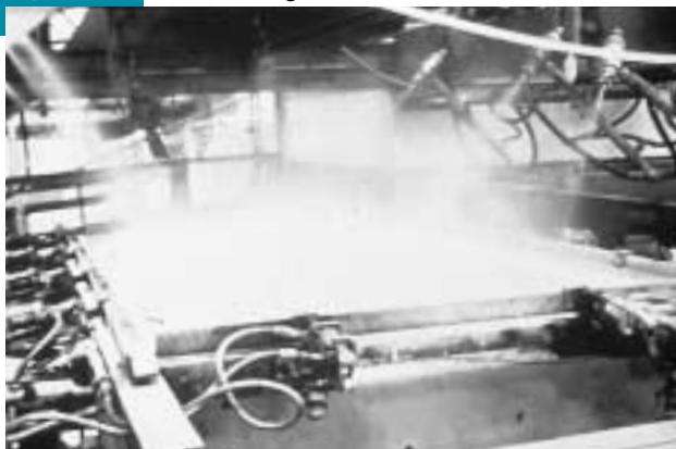
Figure 41 Part Cooling with a Water Mist
