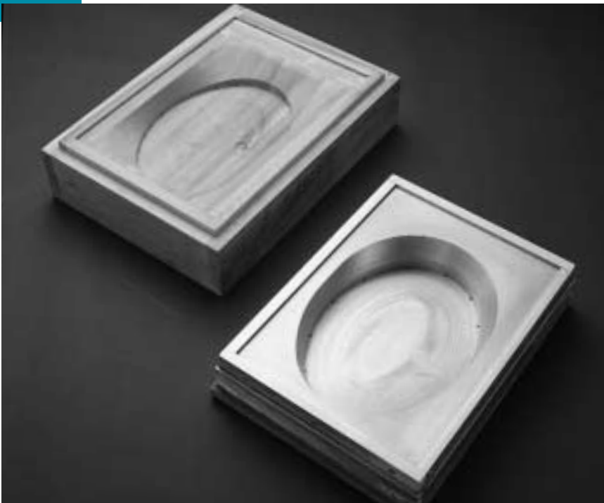
Figure 5 Wood and Aluminum Molds
